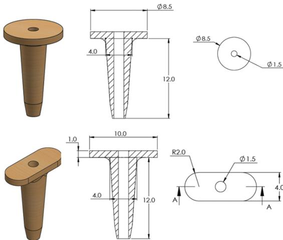
Figure 4. Dimensions of the EnFix TAC products
