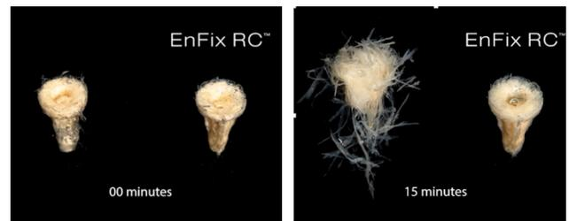
Figure 7. The implant on the left is untreated and loses shape rapidly on immersion in water. Implant to the right is Formlok™ treated.
