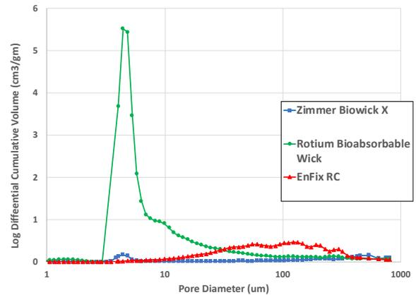
Figure 6. Pore diameter distribution for EnFix compared to competitor products.
