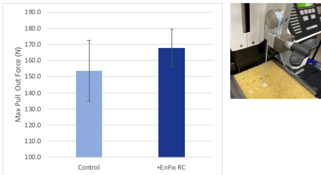
Figure 8. Photograph shows test set up for suture anchor pull out. Chart shows maximum pull out force observed.
